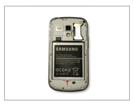
Pull battery out by pulling it up in marked place
