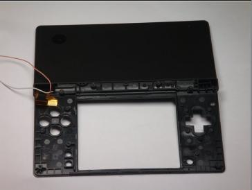
• Flip the case open, and push the lower screen assembly out of the frame.
