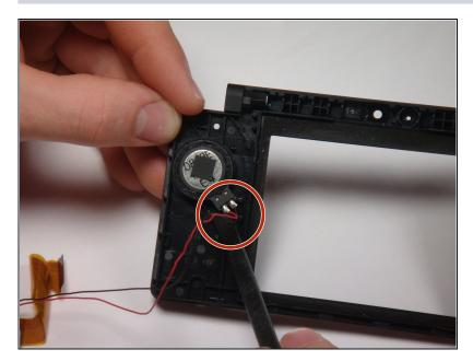
To remove the speakers, place a flat object underneath and gently pry them off.
