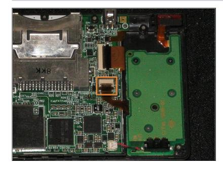
Flip up the black latch and disconnect the D-Pad/Power Button ribbon cable.
