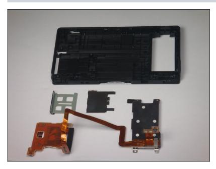
This picture shows the LCD screen, battery compartment, and SD card slot (metal shield and flap) with bottom outer casing.
