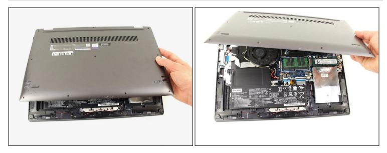
• Once all the clips have been disengaged, lift off the back cover.
