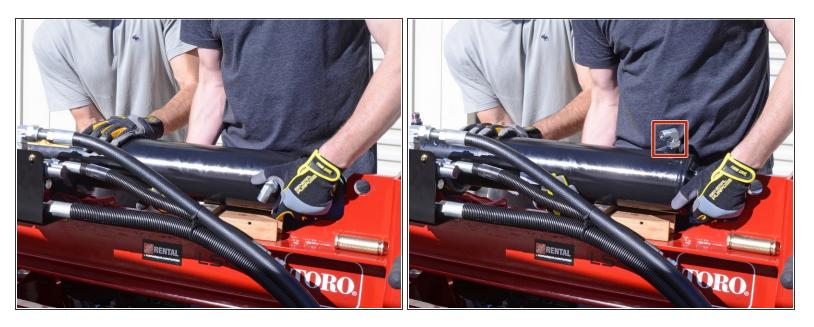
Rotate the cylinder until the L-fitting is vertical.
