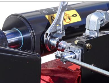
Use an adjustable wrench to loosen the fitting on the cylinder.
