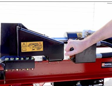
Push the control valve lever towards the rear of the device to extend the piston and advance the cutting wedge.
