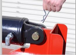
Pull to remove the two cotter pins securing the large pivot pin.
