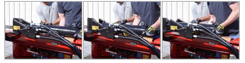
Support the cylinder and push the assembly towards the rear of the device until it clears the dislodger bracket.
