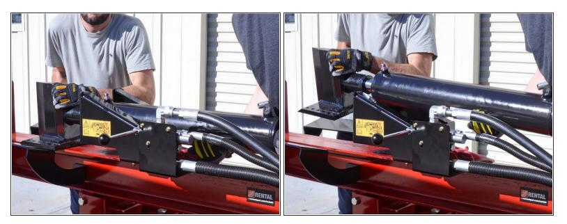
Remove the cylinder and wedge assembly.
