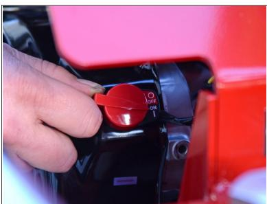
Flip the red engine ON/OFF switch to the ON position.
