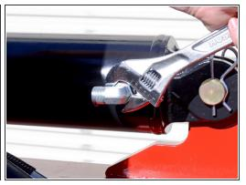
Use an adjustable wrench to loosen the nut securing the L-fitting to the side of the cylinder.
