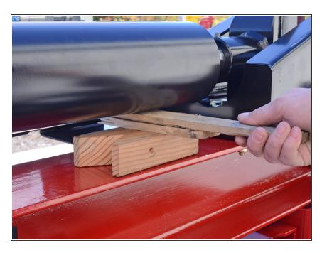
Shim the cylinder with wood blocks to keep it at its resting height, parallel to the frame.
