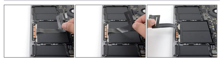
• Carefully peel the trackpad ribbon cable up off the battery, and push it out of the way.
