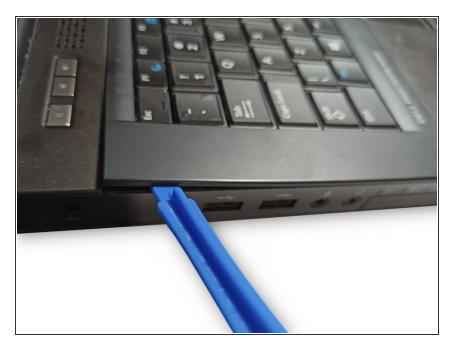
Pry and remove the frame around keyboard (it's a bit lighter than rest of casing).
