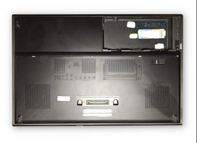
Before any repair, you should remove battery
