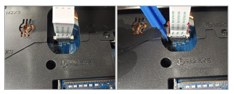
Pry up the white part of connector (constant for both sides) and eject connecting flex
