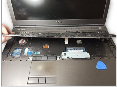
Pick up a little keyboard and eject it. Than pick up harder but DO NOT take it out
