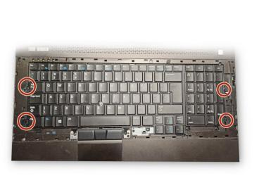
Pry out four hooks which are on the sides of keyboard (two per one site)
