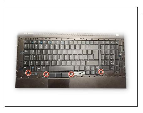
Unscrew 4 fastening screws which are at bottom of keyboard
