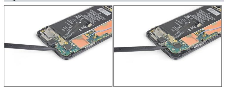
• Insert the tip of a spudger underneath the bottom edge of the motherboard and pry it up enough to grip it with your fingers.
