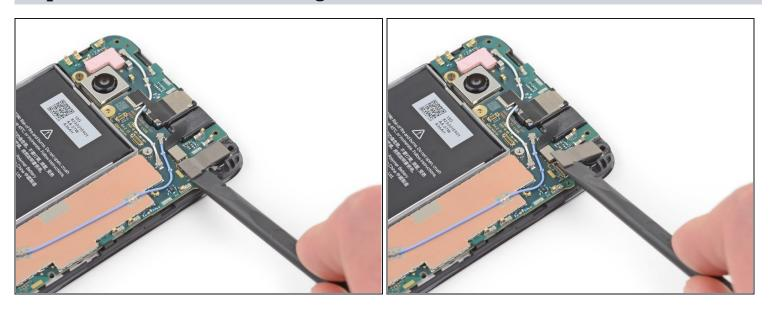
Pry up with the flat end of a spudger to disconnect the front-facing camera from the motherboard.
