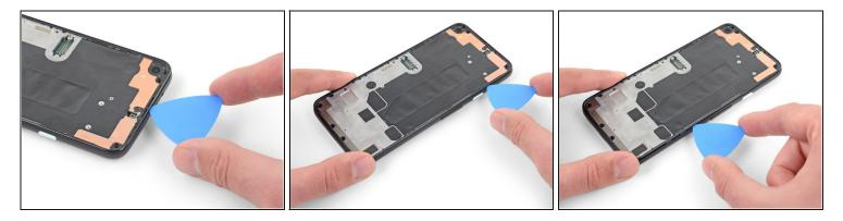
Slide the opening pick around the top and right edges of the phone to release the rest of the clips.
