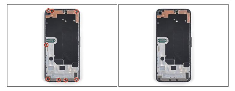
Use a T3 Torx driver to remove the eight 4.3 mm screws securing the back cover to the midframe.
