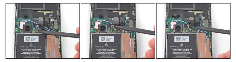
• Use the tip of a spudger to disconnect the two flex cables connecting the fingerprint sensor and buttons to the motherboard.
