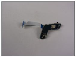
• Locate the IR sensor on the motherboard. Then, use <u>tweezers</u> to gently detach the blue/white ribbon that attaches the IR sensor to the motherboard.
