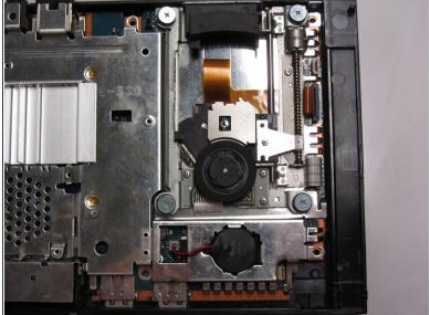
Locate the optical drive on the motherboard.
