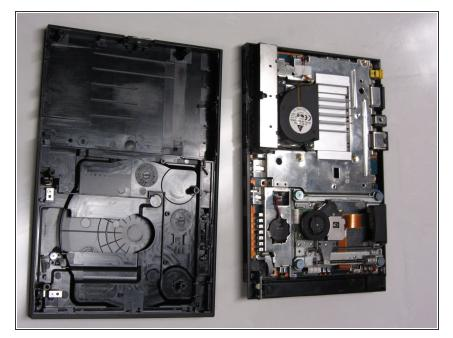
If done correctly, you should have a fully detached plastic backing, revealing the electronic components of the PlayStation 2.
