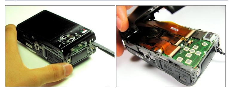
• Use the flat end of a spudger to pry apart the back cover from the rest of the unit as shown.
