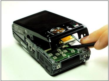
• Using your fingernail or a spudger, flip up the ZIF locking flap on the two LCD ribbon cable sockets that connect the back cover to the rest of the unit.
