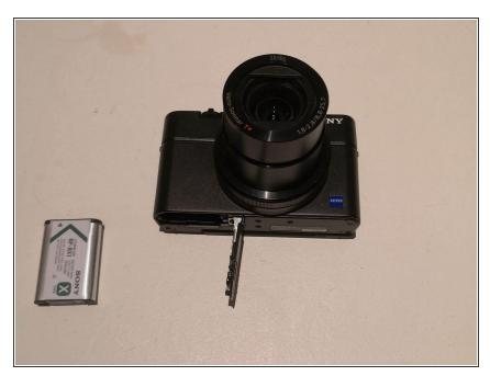
Turn on the camera so the lens comes out. With the lens extended, remove the battery so the camera will not shut down.
