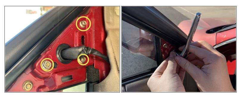
Remove the three 8mm bolts with the socket wrench and 8mm socket header.
