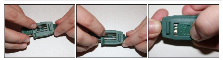
• Carefully insert the working fuse back into the tree plug, and put the cover on.
