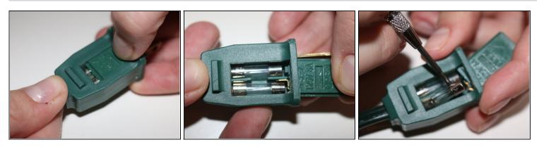
• Open the fuse cover, then use a small flathead screwdriver or spudger to carefully remove the fuse.
