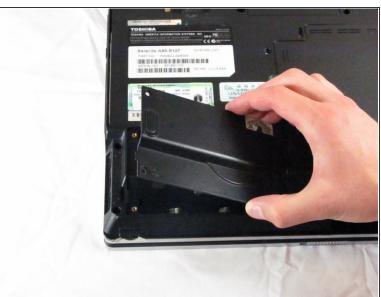
Insert the plastic opening tool into the tab shown and lift up to remove the lower left plate.
