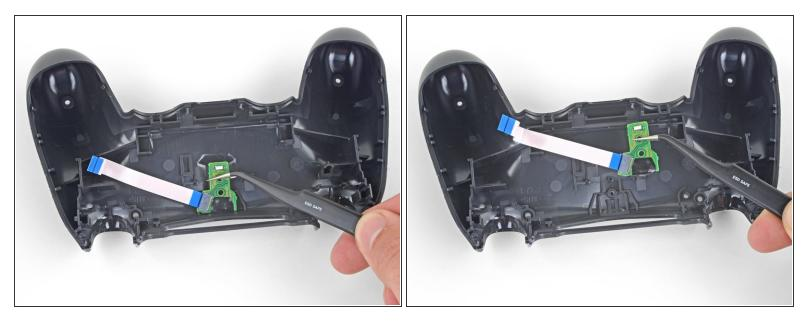
• Use your fingers or a pair of tweezers to remove the charging assembly from the rear panel.
