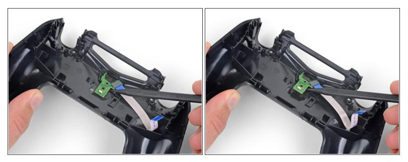
• Use the pointed end of a spudger to lift the charging assembly away from the rear panel.
