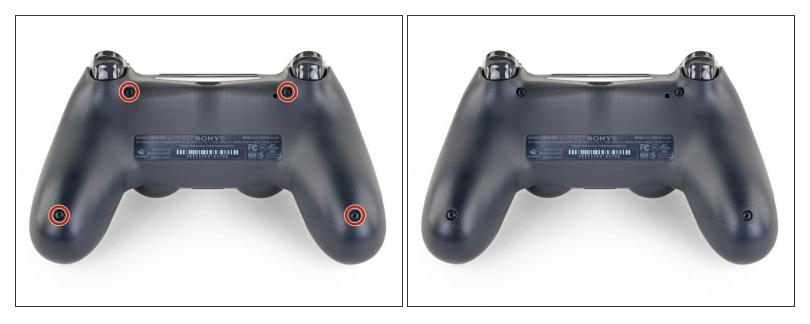
• Use a Phillips screwdriver to remove the four 6.4 mm-long screws from the rear panel.
