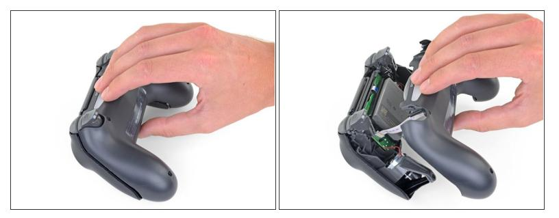
• Lift the rear panel directly away from the controller.
