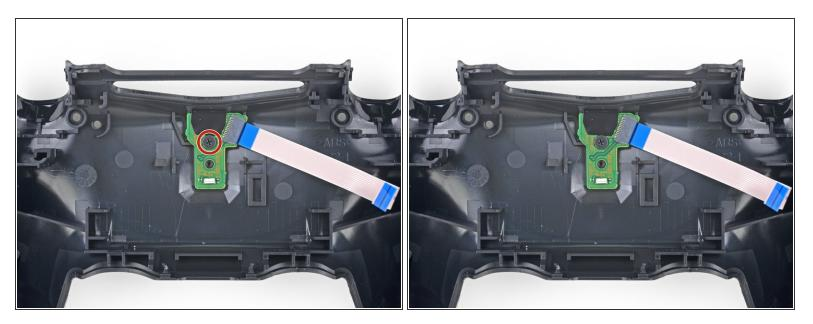
• Use a Phillips screwdriver to remove the 4.4 mm-long screw from the charging assembly.
