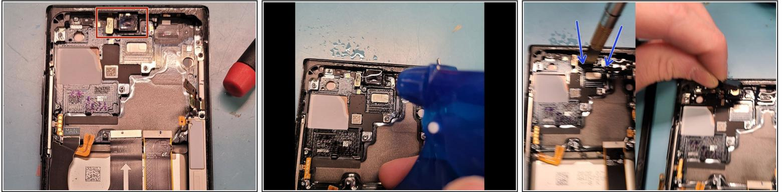
**⚠ Front Camera do not break it is serialized to the phone! Can't be repaired if is broken!**
