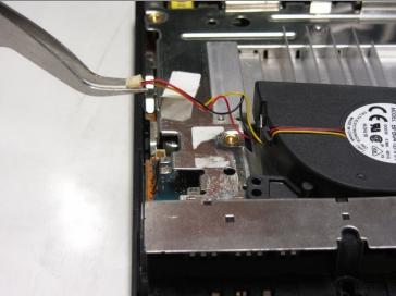
• Detach the terminal (white covering) to the red and yellow cords from the motherboard to the fan with the use of tweezers.
