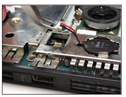
• Identify the clock battery, then use <u>tweezers</u> to disconnect the connector from the motherboard.
