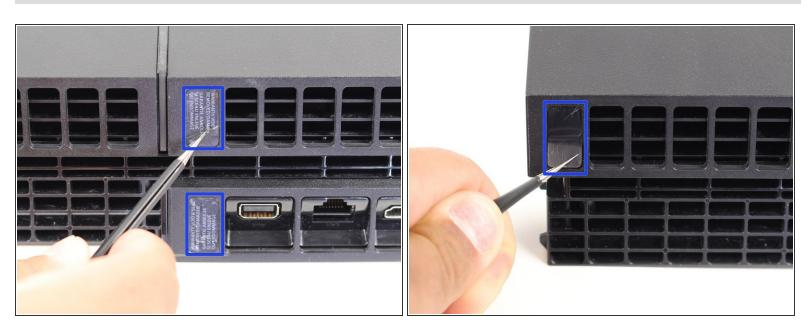
Remove the four stickers on the back of the PS4.
