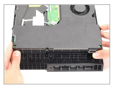
• Lift straight up on the power supply.
