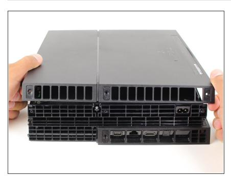
• Remove the bottom panel by lifting the front piece up and sliding the panel towards the back.
