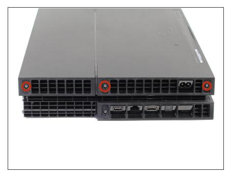
Remove the three 9mm TR8 Torx Security screws on the back of the system.
