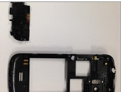
Find the back casing of the phone. Slide the plastic opening tool under the bottom of the speaker to pop it out.
