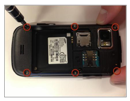
Using a Phillips #00 Screwdriver, remove the six 5 mm screws from the back casing of the phone.
