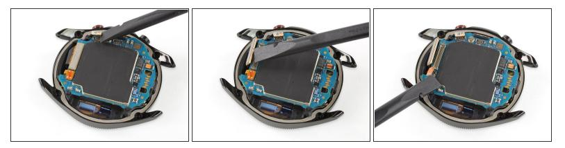
• Use the flat end of a spudger to disconnect the flex cables of the side buttons, the display and the hall sensor.
