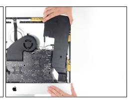
Lift the speaker straight up and remove it from the iMac.
