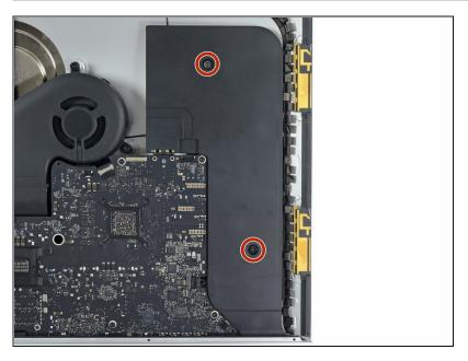
Use a T10 Torx screwdriver to remove the two 10 mm screws securing the right speaker.
