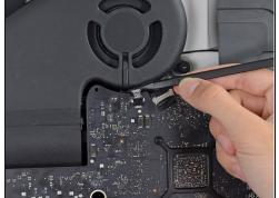
Use the tip of a spudger to disconnect the fan cable's connector from its socket on the logic board.
