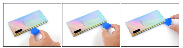
• Slide the opening pick along the left edge towards the bottom left corner to slice the adhesive.
