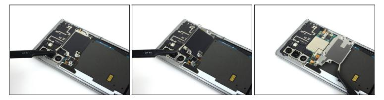
• Use a pair of <u>tweezers</u> to lift up and flip back the metal shield covering the battery connector.
