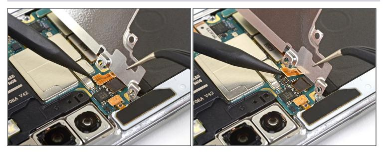
• While holding the metal shield up and out of the way, use the pointed end of a spudger to pry up the battery connector to disconnect it.
