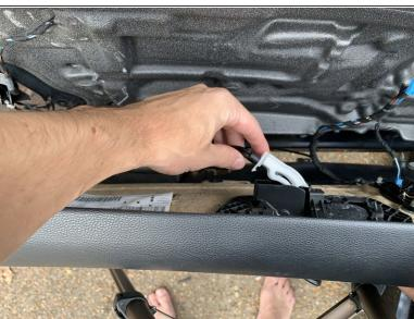
Unclip the internal door handle mechanism inside the door handle by rotating clockwise.
