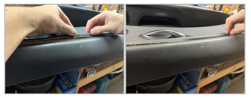
Push the liner into place in between the door panel sections.
