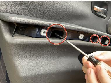
Using a T20 Torx, remove the three screws located behind the previously removed trim.
