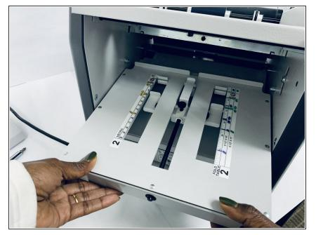
• To remove the second fold table, tilt it upwards and pull it away from the machine to slide it out.
