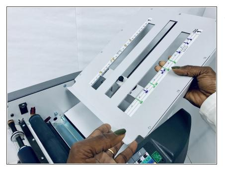
To remove the first fold table, tilt it upwards and pull it away from the machine to slide it out.
