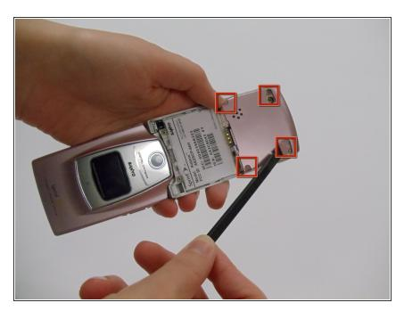
Using a spudger, remove the four rubber coverings on the lower back plate.
