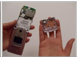
Remove the lower back cover to reveal part of the motherboard and the circular speaker housed in the back cover plate.
