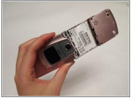
Using a Tri-wing Y0 screwdriver, remove the four 4.4mm screws securing the back plate.
