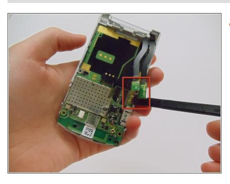
Use the flat end of the spudger to remove two ribbon cables from the back of the motherboard.
