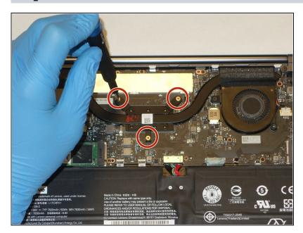
Unscrew the three 3 mm Phillips #0 screws on the heatsink.
