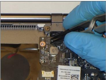
• Using the reverse tweezers, gently pull out the small black cable towards the top right of the motherboard.
