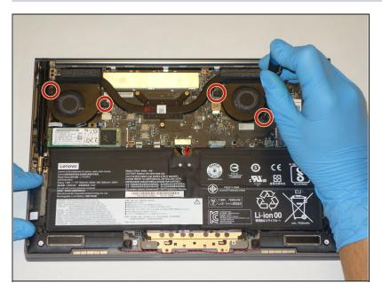
Remove the four 3 mm Phillips #0 screws from the fan assembly.
