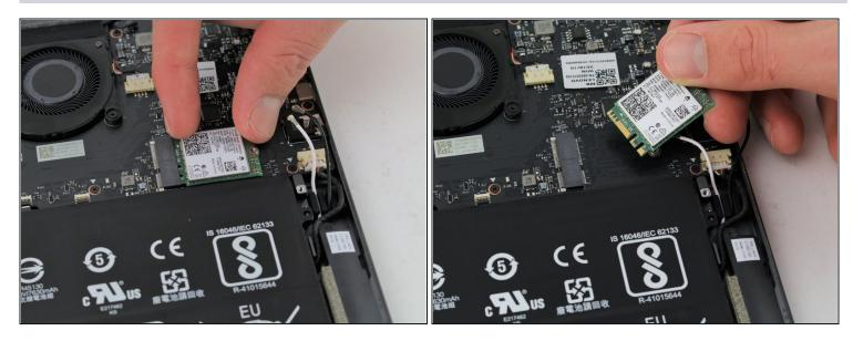
• Pinch the card on either side and pull to the right to unplug it from the motherboard.
