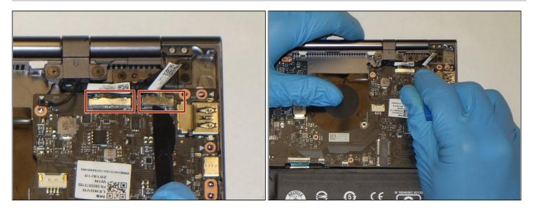
• Using the plastic opening tool, gently pry up on the metal tabs of the two display cables to remove the cables from the top right corner of the motherboard.
