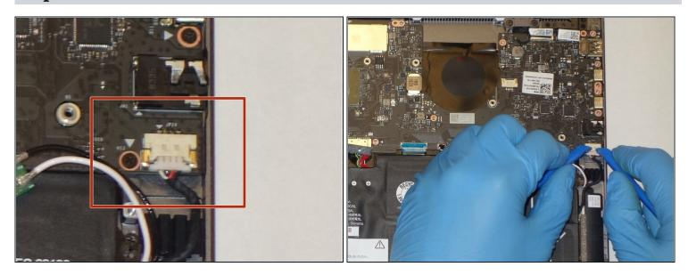
• Using two plastic opening tools gently unplug the white speaker cable connector from the bottom left of the motherboard.
