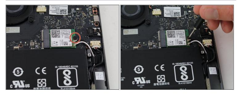
• Use a Phillips #00 screwdriver to remove the single 2 mm screw that attaches the card to the motherboard.
