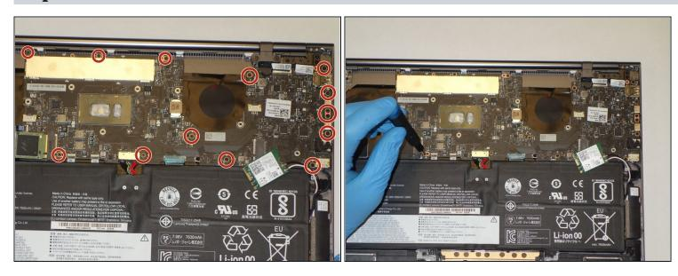
• Remove the fourteen 3 mm Phillips #00 screws that hold in the motherboard.
