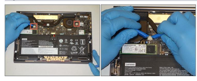
• Use a plastic opening tool to remove the two small, white power cable connectors for each of the two fans.
