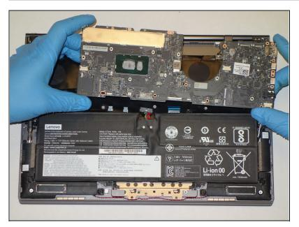
While gently grasping each side of the motherboard, carefully lift the assembly out.
