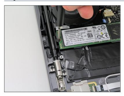
Remove the screw (2 mm with a 5 mm head) that connect the SSD to the motherboard using a Phillips #00 screwdriver.
