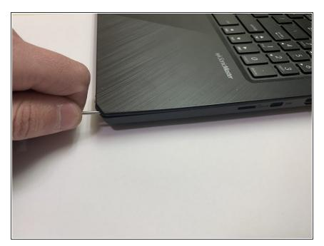
With the laptop open, use a opening tool to detach the keyboard from the laptops body. Lift the keyboard up slowly as to not damage the ribbon cables that connect from the keyboard.
