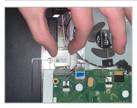
Gently pull the card to the side and it will come out of its socket. The wi-fi card can now be replaced.
