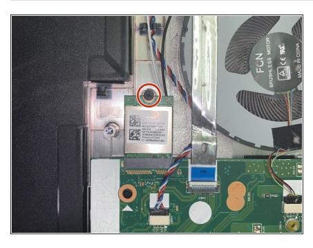
Remove the 3mm Phillips #00 screw securing the card in place.
