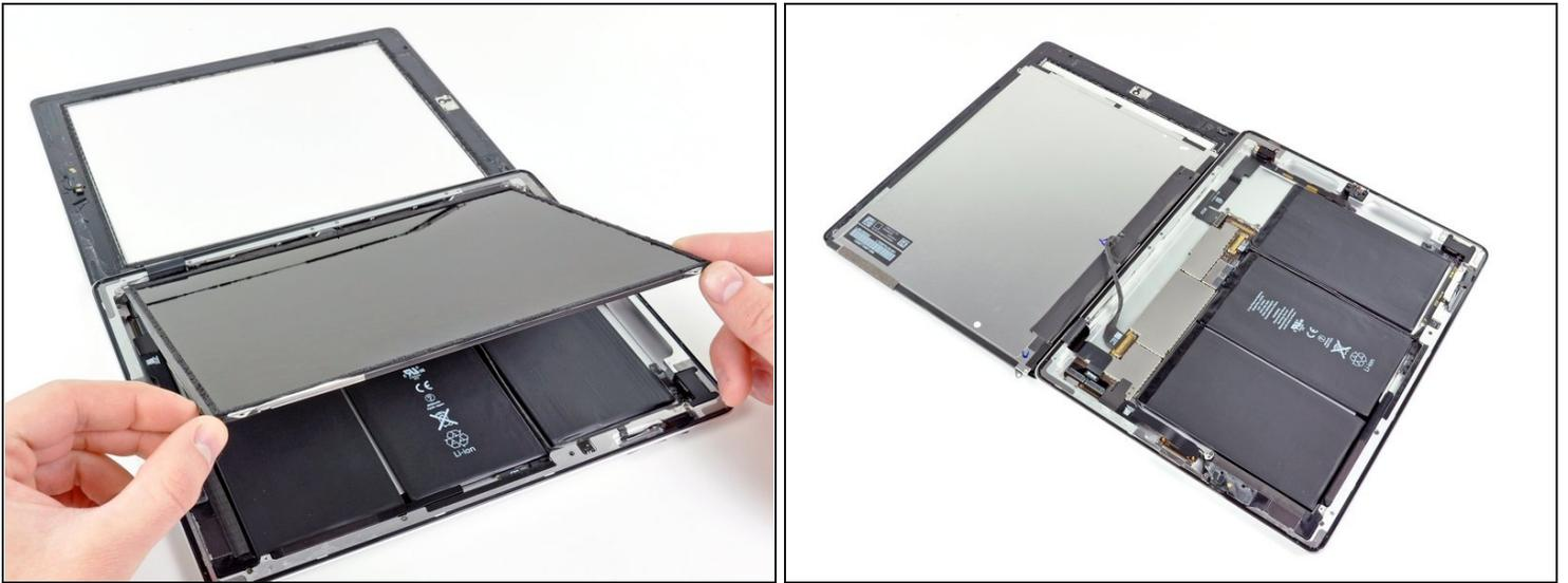
ⓘ The front panel ribbon cables are connected beneath the LCD. To access them, you'll need to temporarily flip the LCD over and out of the way.
