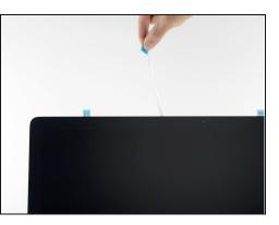
• Remove one side of the protective film from strip 11 by pulling its tab straight up.
