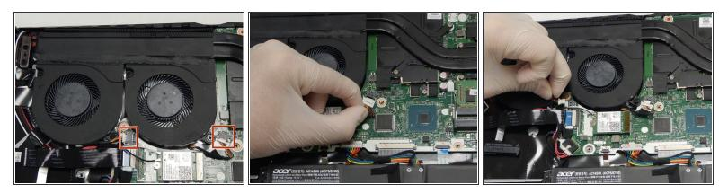
• Using your fingers, slide out the two fan cables from their connectors on the motherboard.
