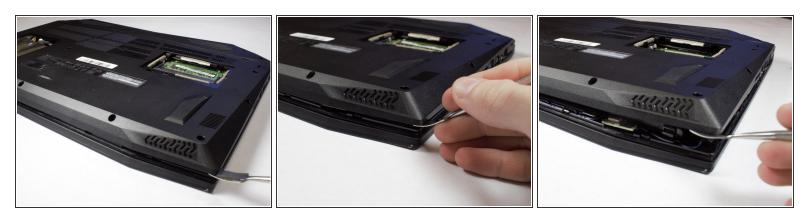
Carefully remove the back shell from the device by prying at the creases with a spudger around all the edges.
