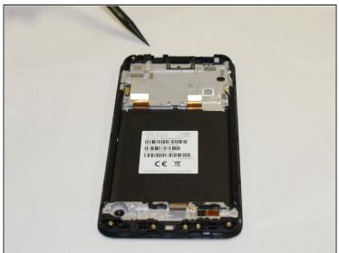
After removing the motherboard and the charging dock, the screen assembly can be replaced.
