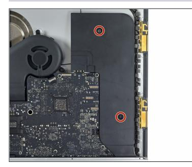
• Remove two 9.8 mm T8 screws.
