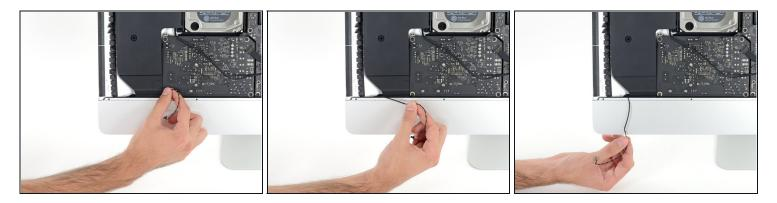
• Gently de-route the power button cable from its groove in the left speaker.
