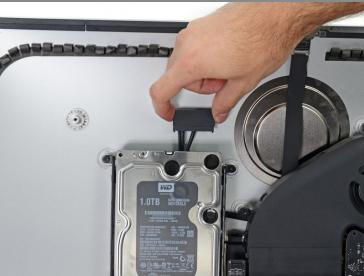
• Pull straight up on the SATA data/power cable to disconnect it from the drive.
