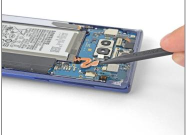
Use the tip of a spudger to disconnect the orange ribbon cable connecting the battery to the motherboard.
