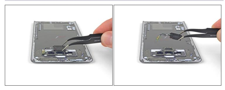
• Remove the fingerprint sensor.
