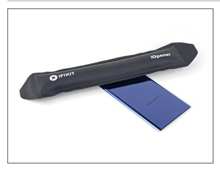
Use a heat gun, hair dryer or apply a heated iOpener on the outside of the fingerprint sensor to soften the adhesive underneath. Heat it until it's slightly too hot to touch, as the adhesive is soft and resists tearing.
