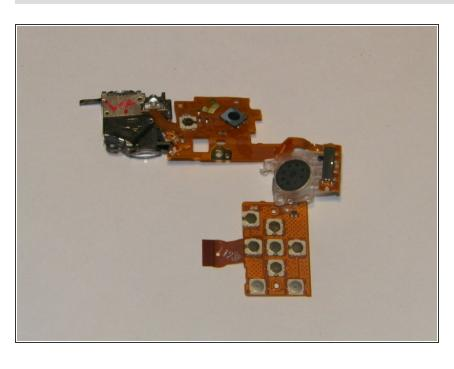
The rear control board should now be completely separate from the camera. To reassemble your device, follow these instructions in reverse order.
