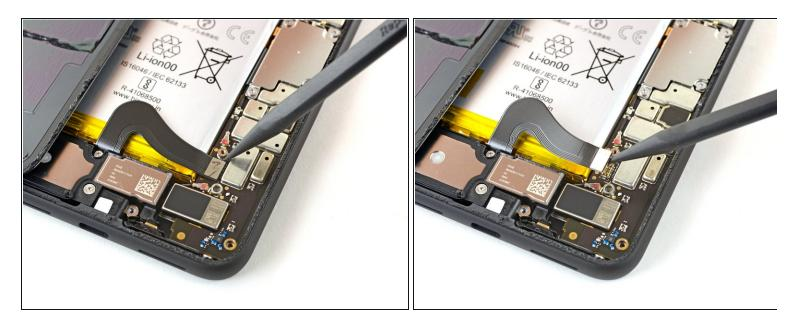
Mhenever you use the spudger near the battery, be very careful not to puncture the battery.
