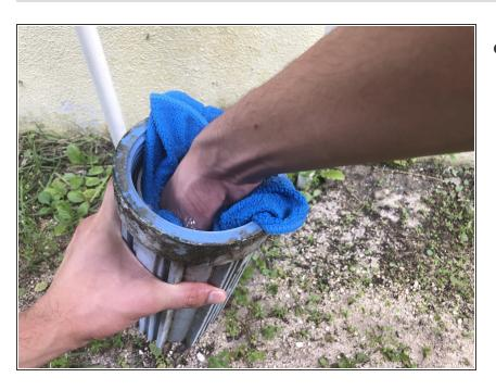
Clean out the inside of the filter canister with soap and water.
