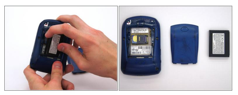
• Remove the lithium-ion battery from the back of the device using your index finger.
