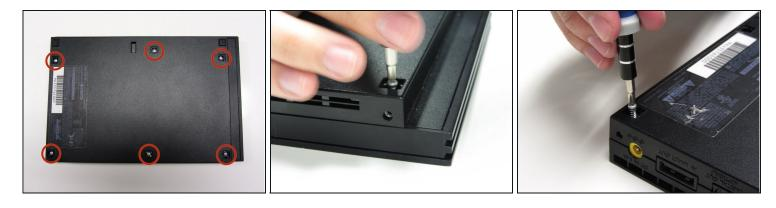
• Remove all six 4.0 mm screws from the base of the unit using a #1 Phillips screwdriver.
