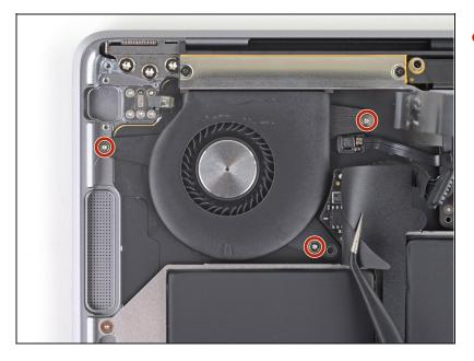
Use a T5 Torx driver to remove the three 2.7 mm screws securing the fan.
