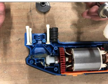
Remove the pendulum and recover the bearing.
