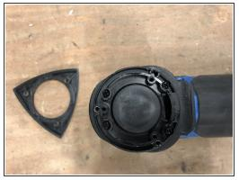
Replace the holding flask, be careful to have the three small balls.
