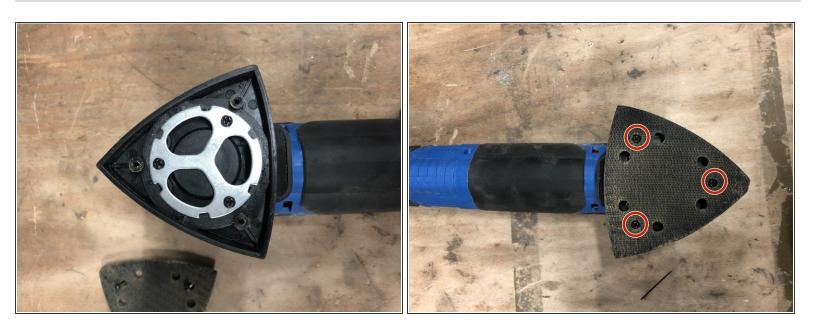
• Line the three screws of the holding flange and then that of the pad.
