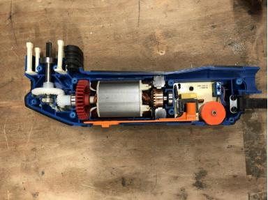
Unscrew the screws to open the shell.
