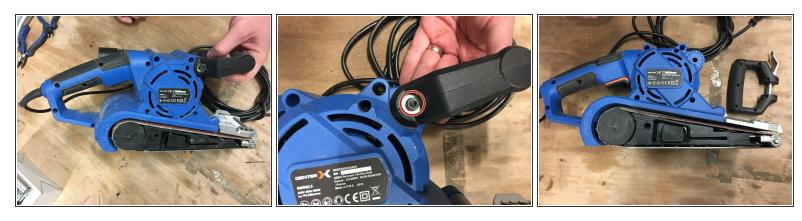
Remove the handle by unscrewing the screw.
