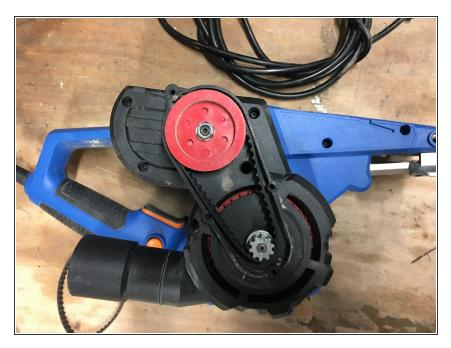
Replace with the new drive belt. To put it on, place the drive belt on the right wheel first.
