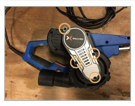
Unscrew the four screws to access the drive belt.
