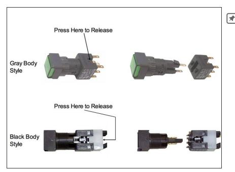
For reinstallation, locate the white dot on the exposed surface, and line this dot up with the slot in the middle of the button. Press the button straight in.
