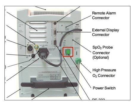
Use a pair of slim pliers or tweezers to grip the cap of the power switch button. Pull it straight out.
