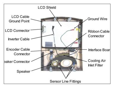
Disconnect the three tubes from the barbed fittings along the bottom of the inside of the front enclosure. Be sure to note where they were connected.
