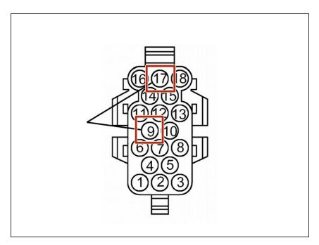
Switch terminals are connected to pins 9 and 17 shown, regardless of the O2 pressure switch type.
