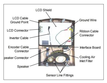
Turn the unit off and disassemble the front enclosure (previous steps).
