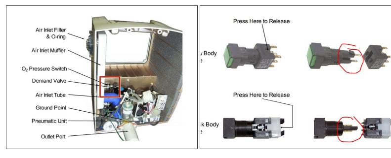
For the brass colored metal located on the back wall of the rear enclosure, connect the ohmmeter to the two tabs located on the back of the switch body.
