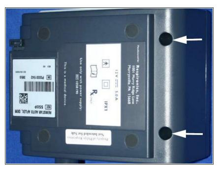
Remove the top cover by using a Torx T15 to remove the 2 screws on the back of the enclosure.
