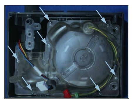
Remove the Blower Cap by using the T8 Torx screwdriver to remove the 7 screws that secure the Cap to the enclosure.
