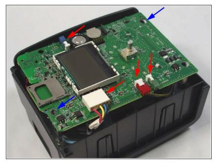
Remove the Main PCA by removing the wiring harnesses and squeezing the 2 standoffs in the corners of the board.
