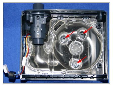
• Align the stands located on the bottom of the blower assembly with the holes in the blower housing.
