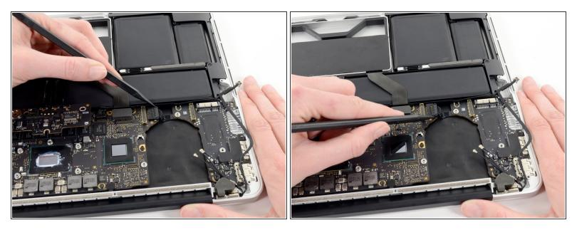
Use the tip of a spudger to push the edges of the I/O board power connector straight out of its socket on the logic board.
