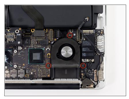
Remove the three 3.1 mm T5 Torx screws securing the right fan to the logic board assembly.
