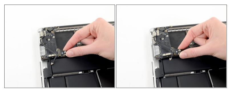
• Carefully pull and remove the I/O board away from its recess in the upper case.
