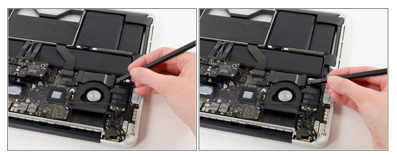
Use the flat end of a spudger to pry the right side of the I/O board data cable connector up off its socket on the I/O board.
