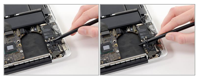
Move the antenna cables aside, clear of the AirPort board.
